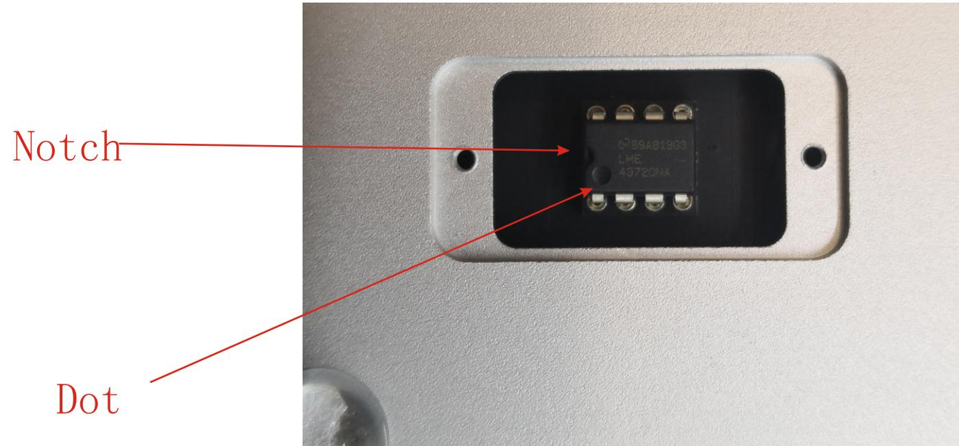
Make sure the notch and dot of the LME49720 are on the same side with the notch of the socket.
