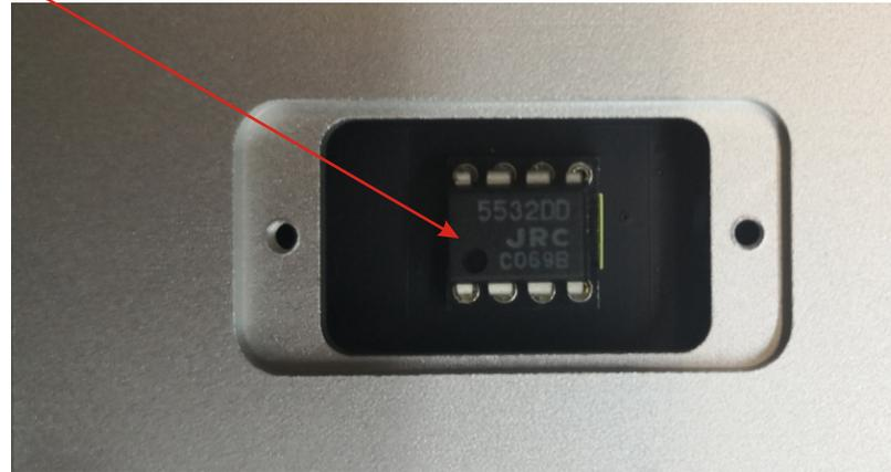
Make sure the dot of the NJM5532 are on the same side with the notch of the socket.
